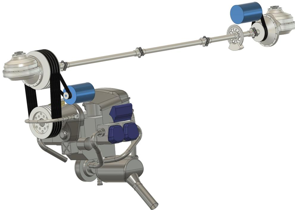
Figure 9.2: Front-left isometric view of engine and transmission
