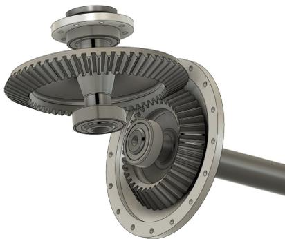
(b) Bevel gear meshing
